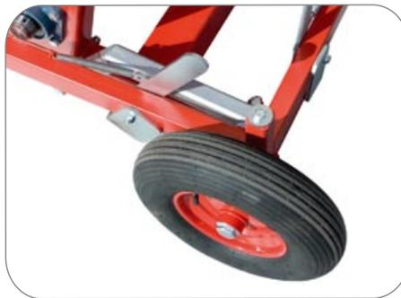
2 off. Polyurethane-filled rubber wheels
