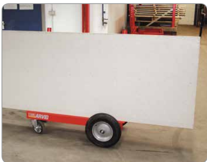
A versatile transport trolley for board material.
